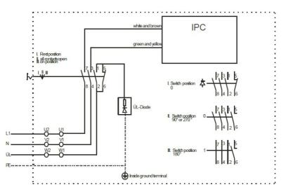
Figure 4. Display of the server's connection to the power grid
