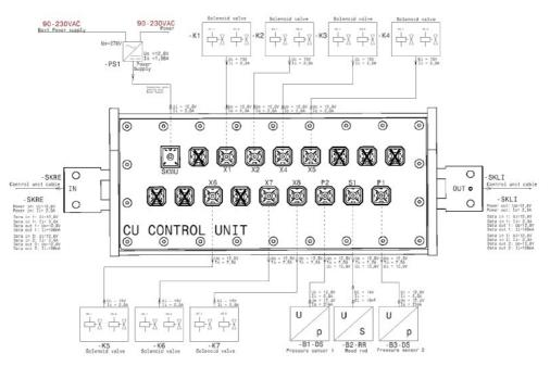
Figure 8. Connection diagram of the SCU control unit
